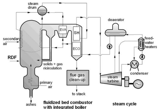
Fig. 5. Configuration of fluidized bed combustor considered for strategies 3 and 4. In large plants, a section of the economizer is placed ahead of the superheater to limit the temperature of the gas entering the superheater to 650 °C.
