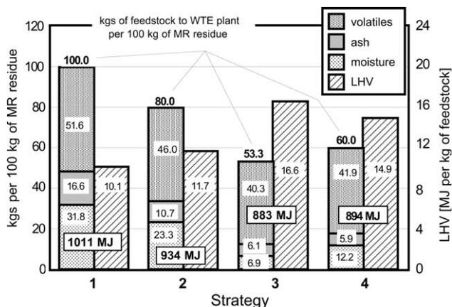
Fig. 3. Characteristics of the feedstock supplied to the WTE plant. The LHV bars (to be read on the right vertical axis) give the heating value specific to 1 kg of feedstock supplied to the WTE plant. Instead, the MJ within boxes are the total LHV supplied to the WTE plant per 100 kg of MR residue.
