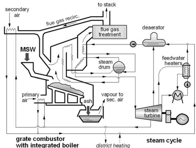
Fig. 4. Configuration of grate combustor considered for strategies 1 and 2. The extraction of steam (at 2.6 bar) for district heating is considered for the large plant of strategy 1 to assess the cogeneration of power and heat. In the large plant of strategy 2, a section of the economizer is placed ahead of the superheater to limit the temperature of the gas entering the superheater to 650 °C.
