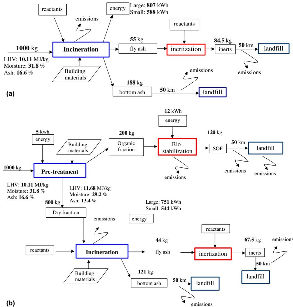
Fig 2. (a) Schematic representation of strategy 1, with basic mass and energy flows for 1 metric ton of MR residue. (b) Schematic representation of strategy 2, with basic mass and energy flows for 1 metric ton of MR residue. (c) Schematic representation of strategy 3, with basic mass and energy flows for 1 metric ton of MR residue. (d) Schematic representation of strategy 4, with basic mass and energy flows for 1 metric ton of MR residue.
